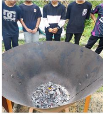
Gambar 6. Proses Pirolisis Biochar.
