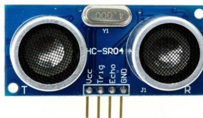
Gambar 2. Sensor Ultrasonik
