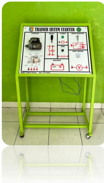
Gambar 2. Trainer sistem starter.
